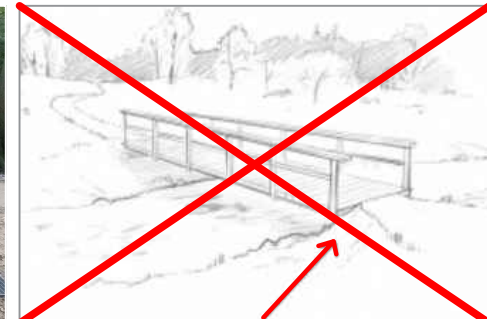
Nogāzes izskalošanās pie tilta pamatnes [Avots: Y. Lundell, 2005. Access to the forests for disabled people]
